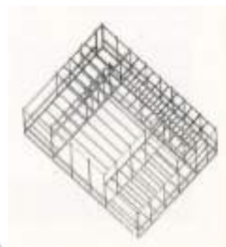
FIGURE 09 » Timber house construction system, extracted from the book Framed Buildings of England by R.T. Manson, 1974.
